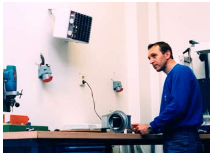
Cat is equipped with a mounted wall bracket that gives the heating fan a tilt angle of 10° for good heat distribution.
